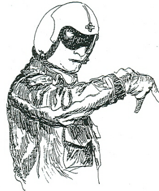
Landing Lights Off
